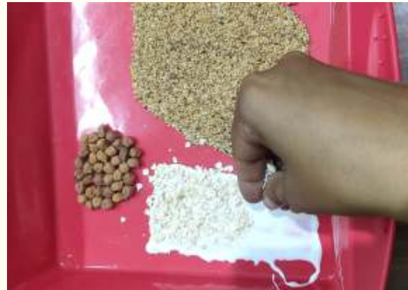
Fixing samples in epoxy resin
